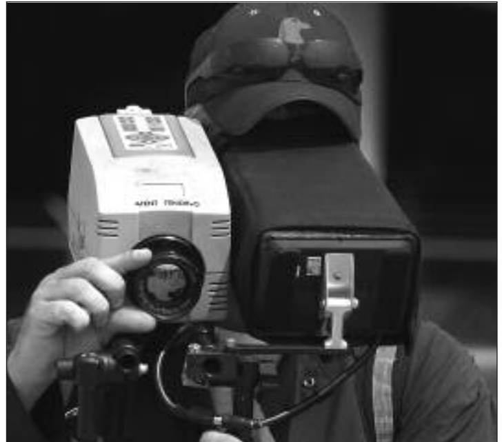
This hand-held Hawk Leak Detection device can spot leaking chemical vapors for tanks, pipelines, barges, railcars and other hazardous chemical containers. Louisiana environmental officials plan to use the machine in the Baton Rouge area ozone non-attainment area.
