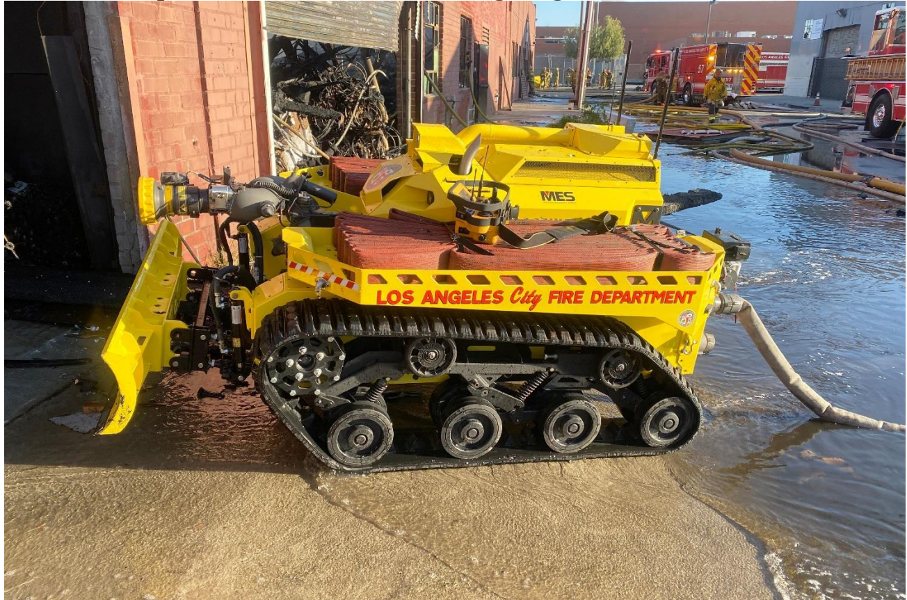
The Los Angeles City Fire Department deploys a human-controlled firefighting machine called Robotics Systems 3. Credit: Captain Robert Barna Los Angeles City Fire Department
